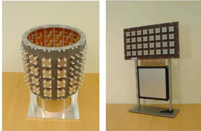
Figure 2.4: A uniform cylindrical array with 128 dual-polarized antennas corresponding to 64 elements (left) and a uniform planar array with 64 dual-polarized antennas corresponding to 32 elements (right) [58].
