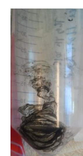
Figure 3. Concentrated AgNP precipitate after freeze drying.
