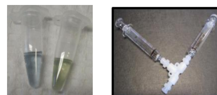
Figure 4. Resuspended AgNP (left) and syringe system (right) used for hydrogel preparation.
