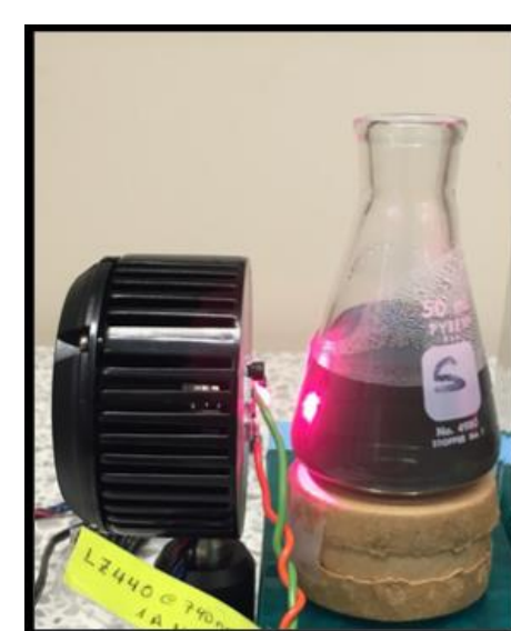
Figure 2. Irradiation of AgNP using an LED.
