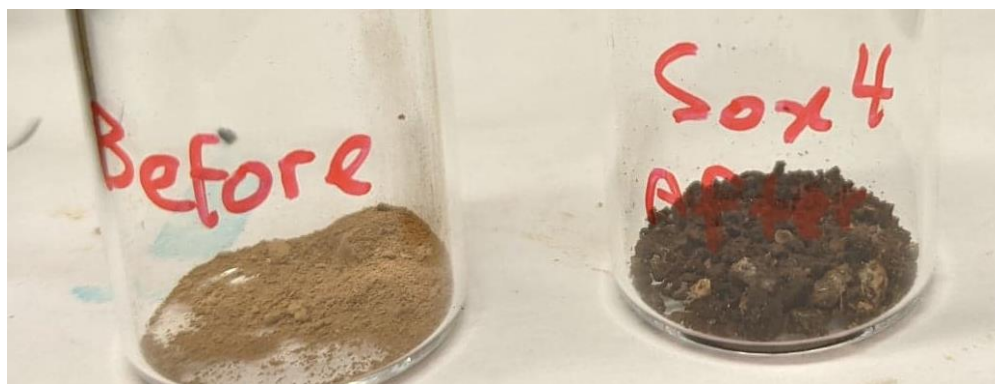
Figure 2.7: On the left: Hinton A protolignin obtained from FP Innovations; on the right: extracted technical lignin via Soxhlet4, with AcN.
