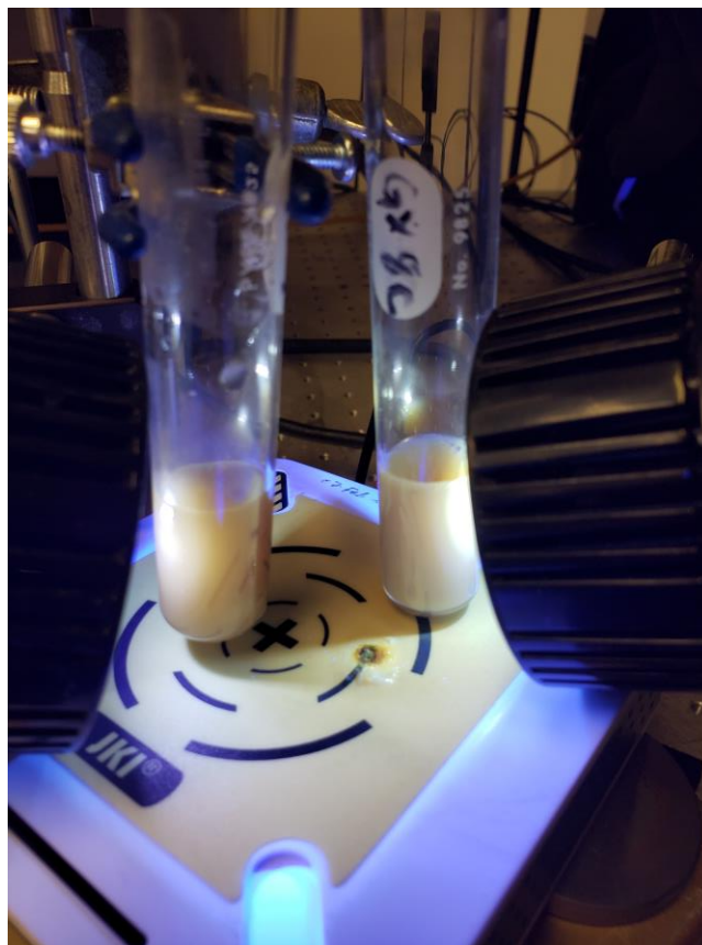
Figure 2.21: LED irradiation setup for protolignin valorization reactions.
