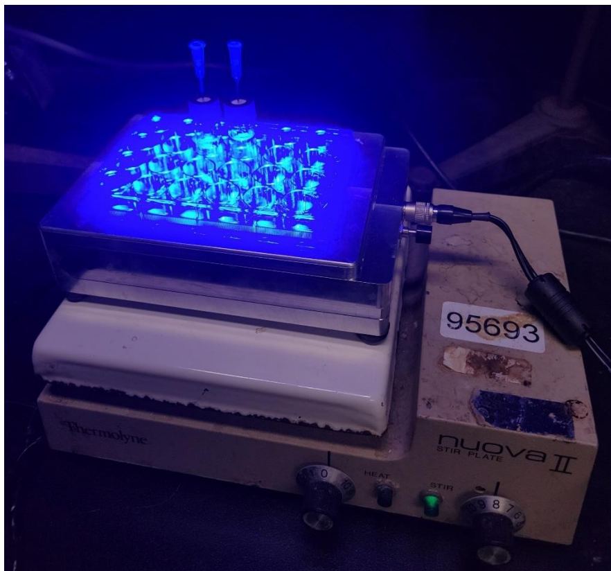
Figure 3.7: Setup for rapid screening of conditions for the photocatalytic cleavage of lignin molecular models using blue light irradiation of a well plate illuminator.
