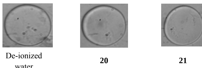
Figure 5.7 Ice crystals of analogues of distilled water (left), 20 (middle) and 21 (right), at 10 mg/mL, as determined by nanolitre osmometry.
