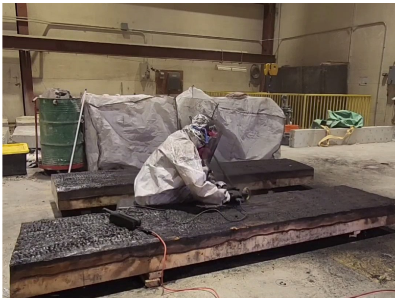
Figure 3-9 Specimen condition: (a) prior to char removal (b) dust removal (c) after char removal using wire wheel brush
