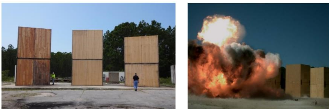
Figure 2-4 Full scale blast test for CLT structures before and after air blast (USACE Protective Design Center Omaha District, 2018).
