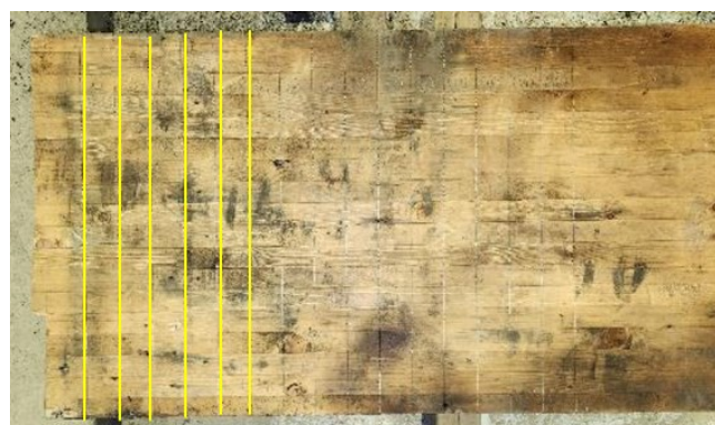
Figure 3-6 Location of the cuts made in the charred GLT specimen along the panel length
