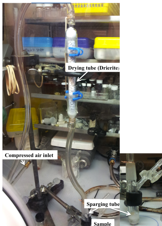
Figure 3.5 Glovebox apparatus used to sparge dry air through a solution of H 2 IMes 3 in C 6 D 6 . All hose attachments are secured with copper wire.
