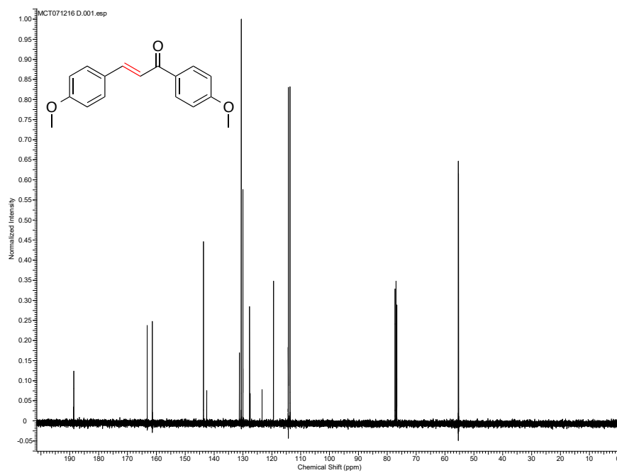
Figure 2A.21. ^{13}\text{C} NMR of 5 Product in \text{CDCl}_3 .
