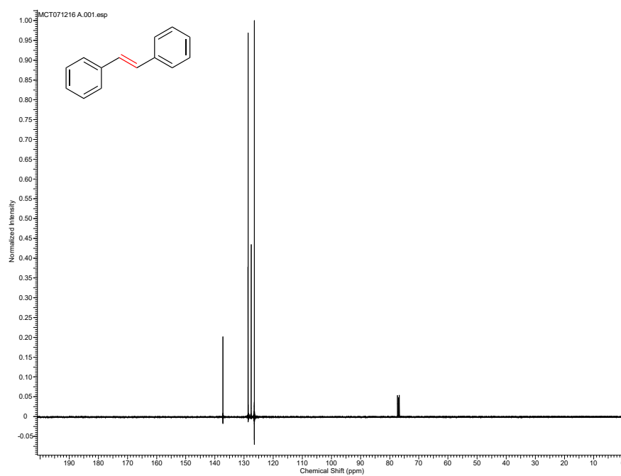
Figure 2A.7. ^{13}\text{C} NMR of 1 Product in \text{CDCl}_3 .
