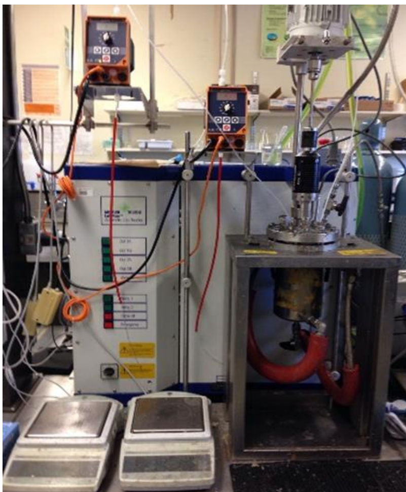
Figure 3.1 Stainless steel LabMax™ reactor (Mettler Toledo).
