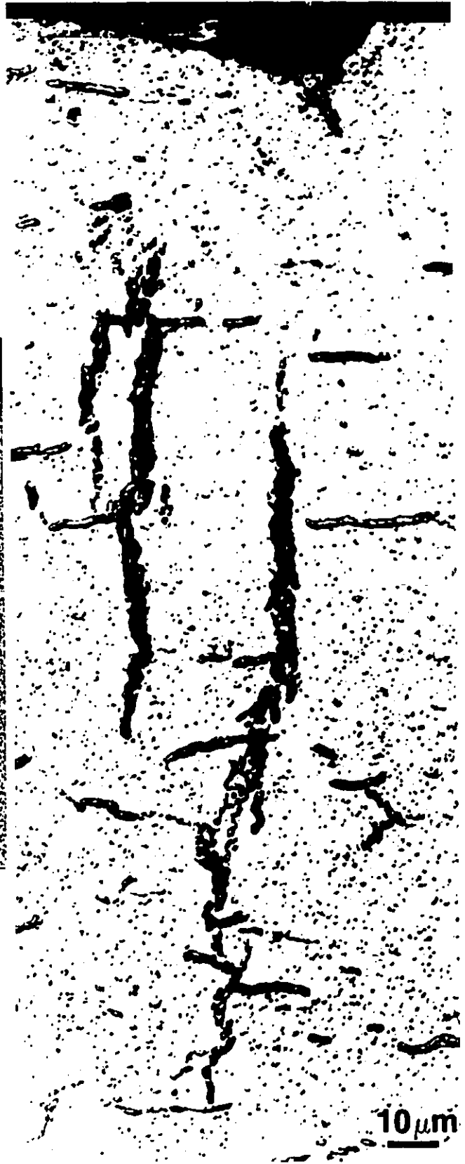
Figure 32 Hydrides Beneath the Notch Near the Edges of a Cantilever Beam Specimen.
