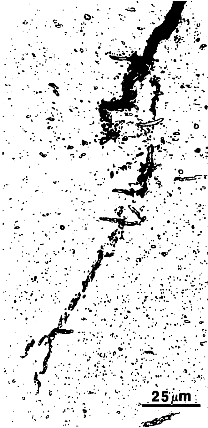
Figure 27 Appearance of Crack-Tip Hydrides in Specimen C148-A22. Note that the crack-tip hydride is comprised of an aligned accumulation of smaller hydrides.
