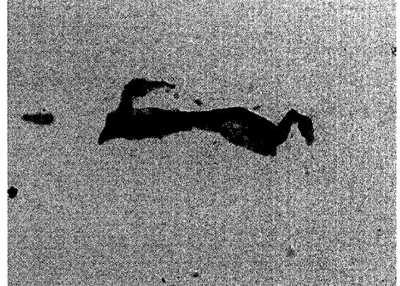
Figure D.27: 85°C MW B, methyl blue staining, 177\ \mu\text{m} < \text{particles} < 420\ \mu\text{m} , 200x.
