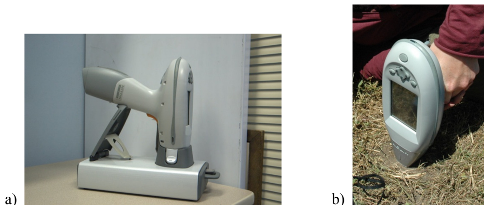
Figure 11 Field-portable X-ray fluorescence analyzer. a) Laboratory use; b) Field use.
