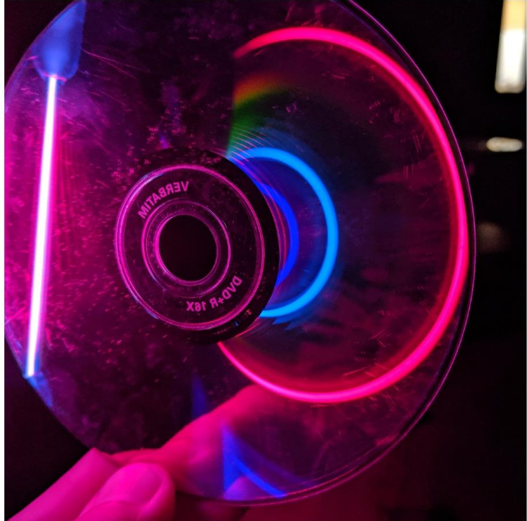
Figure 3 a) Energy-level diagram for hydrogen, colour added from b) to the appropriate transitions. [5] b) Hydrogen lamp and its emission separated by wavelength after diffraction through grooves of DVD. [6]
