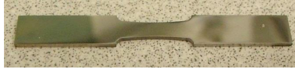
Figure 49: A polished titanium tensile specimen; note the shiny and reflective surface
