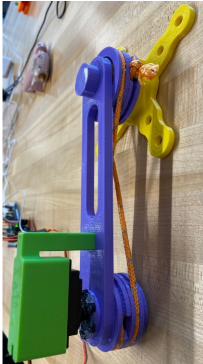
Figure 4-40: 3D Printed Prototype of LMPHJ
