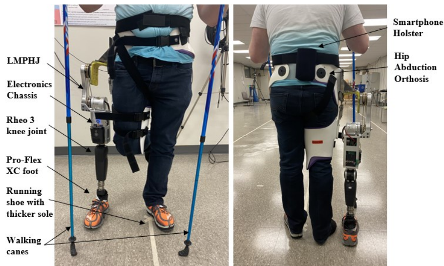
Figure 6-1: Test set-up for LMPHJ evaluation with able-bodied participants
