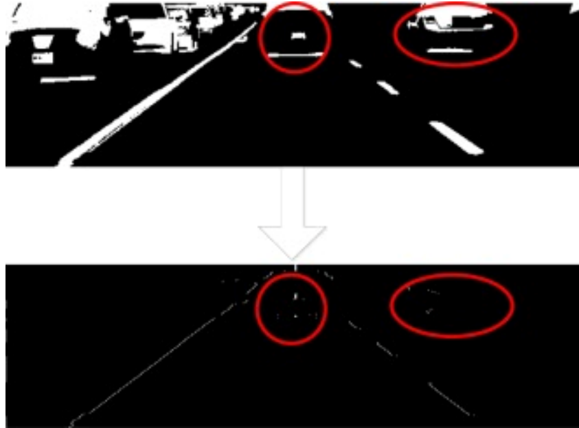
Figure 3.13: Drawbacks of the proposed scanning rule: blobs between line markings and outside the current lane.
