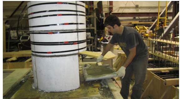
Figure 2-23 Placement of cement paste between concrete raiser units and columns
