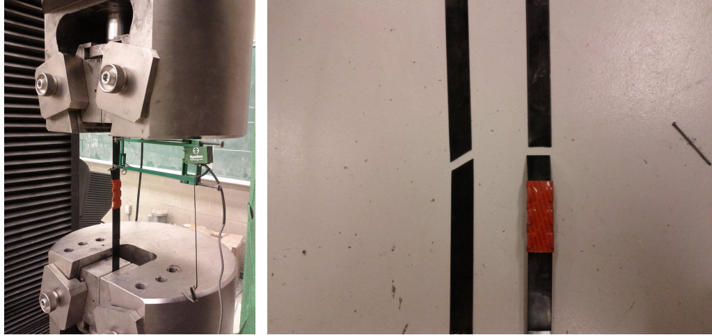
Figure 2-30 From left to right: Galdabini testing machine, and Coupon Types 1, and 2 after the rupturing of steel.
