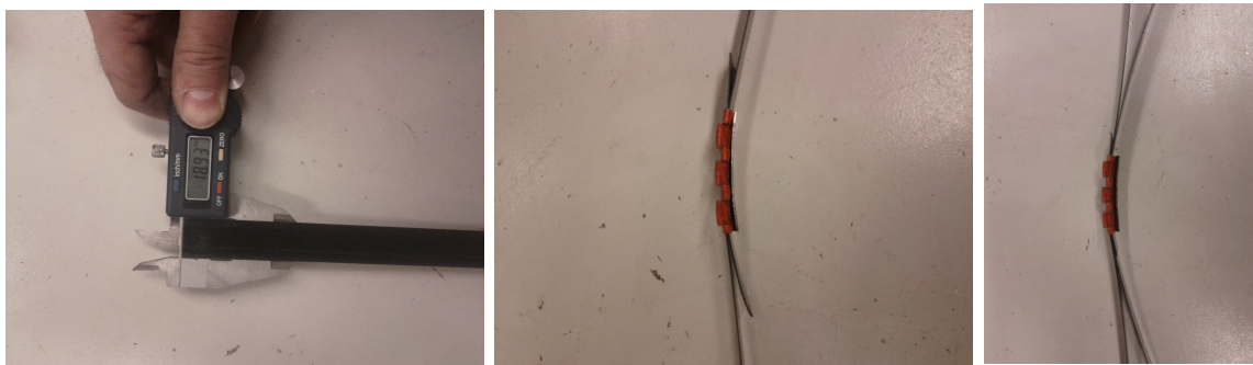
Figure 2-29 From left to right: Coupon Type 1 - Solid Strap (no sealer), Coupon Type 2 - Two straps connected by a sealer, and Coupon Type 3 - Three straps connected by a sealer
