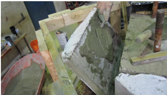
Figure 2-23 Placement of cement paste between concrete raiser units and columns
