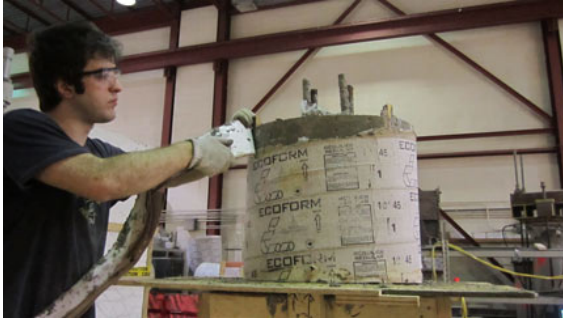
Figure 2-21 Opening of sonotubes after one week
