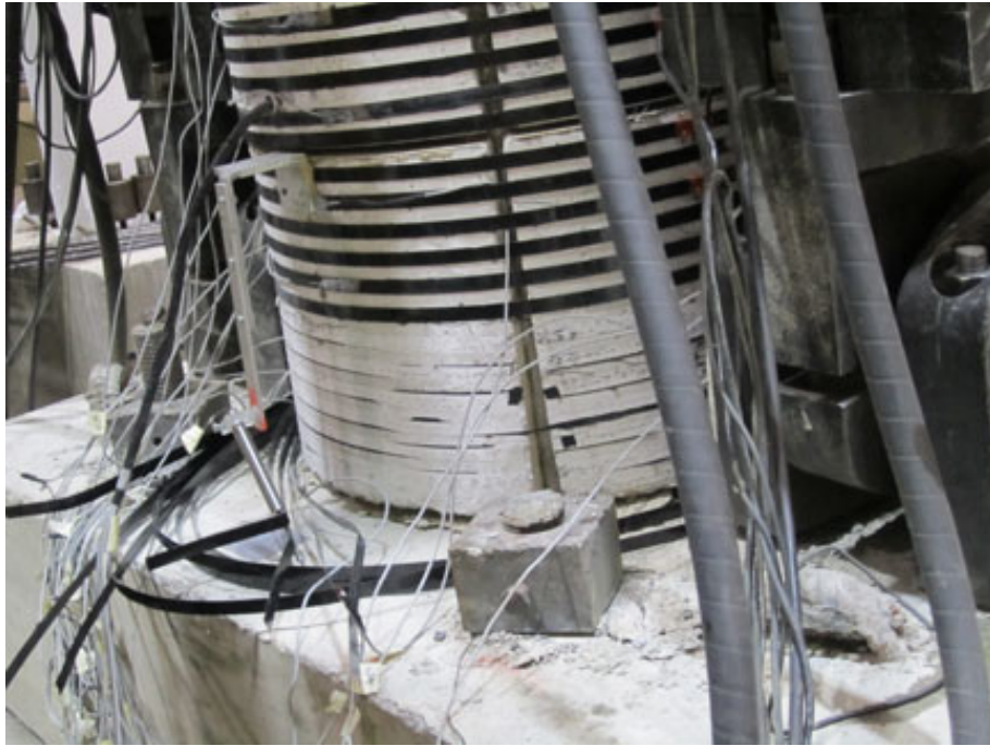
Rupture of 6 strap after first push at 7% drift
