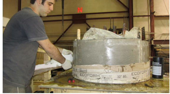
Figure 2-21 Opening of sonotubes after one week
