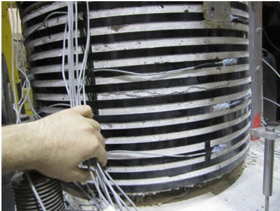
Expansion of cracks on the concrete raiser units after 5% drift
