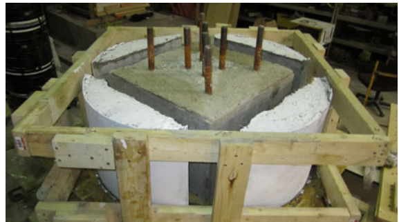
Figure 2-22 Removing the concrete raiser units out of the formwork
