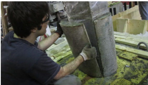
Figure 2-22 Removing the concrete raiser units out of the formwork
