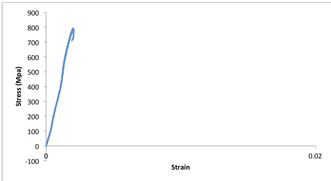
Figure 2-33 Stress-strain relationship of Coupon Type 3 (Three straps connected by a sealer)
