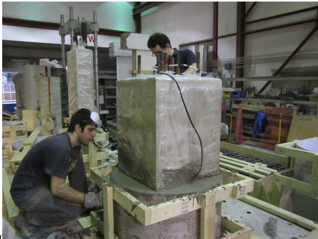
Figure 2-18 Casting of the first layer of concrete raiser units for square column
