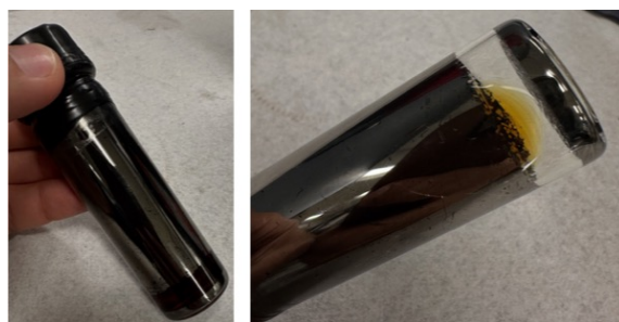
Figure 44. Formation of nickel black due to thermal decomposition of the Ni(cod) 2 at 60 °C
