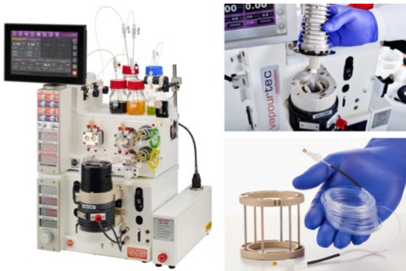
Figure 35. UV-150 photochemical reactor developed by Vapourtec company
