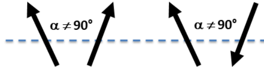
Figure 1.2. Ferromagnetic (left) and antiferromagnetic (right) spin interactions where the spin projections are canted by an angle \alpha within a horizontal axis (dashed blue line).
