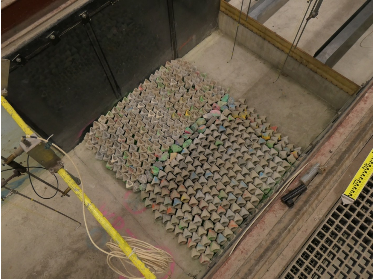
Fig. A2. Eco-friendly submerged breakwater case (TSCC) view no.1
