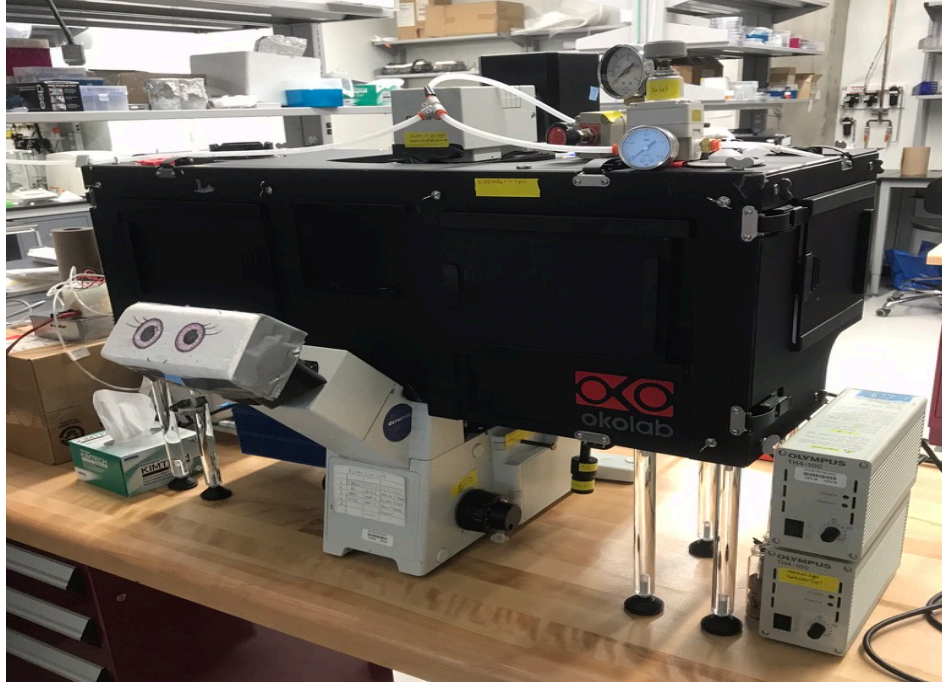
Figure 4-2: Microscope set-up to monitor on-chip elution via fluorescence.
