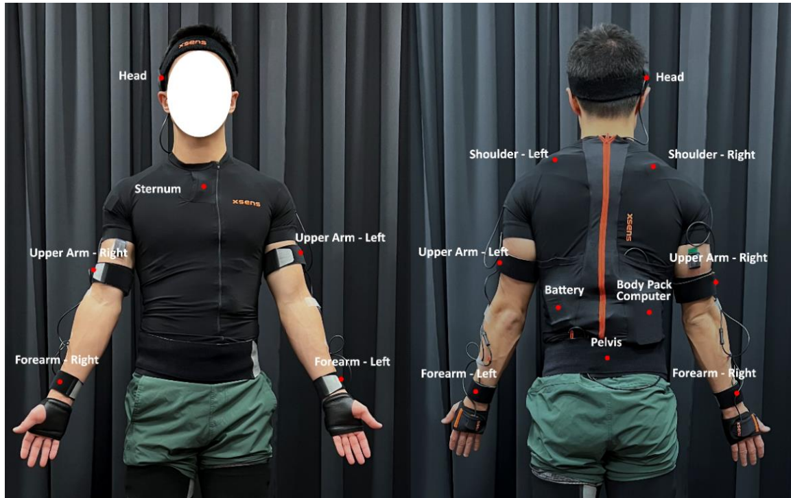
Figure 3. Xsens suit configuration with sensor placement. An upper body configuration (red dot) was used in this study for an upper body model without hands.
