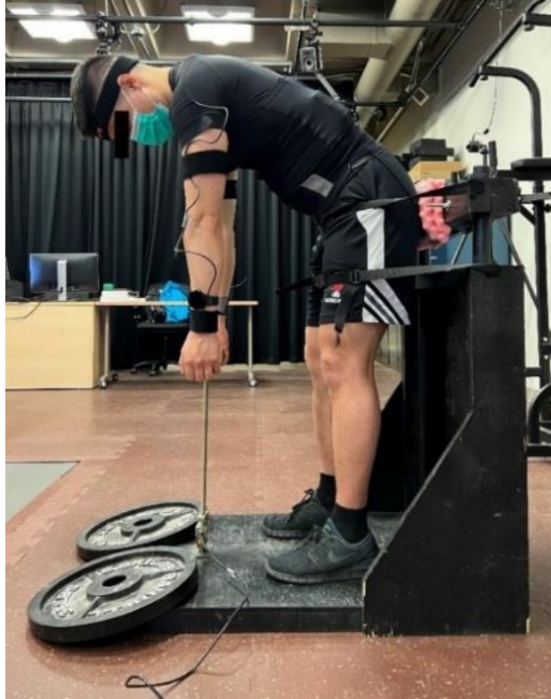
Figure 5. Participants perform the maximum pulling strength test where they are strapped at the pelvis and thigh. The handle of the load cell is adjusted to their knee height.
