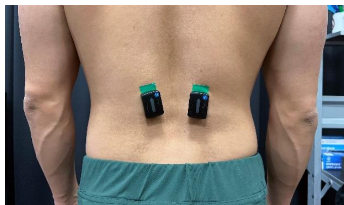
Figure 2. Surface electromyography sensor placement on the left and right erector spinae.
