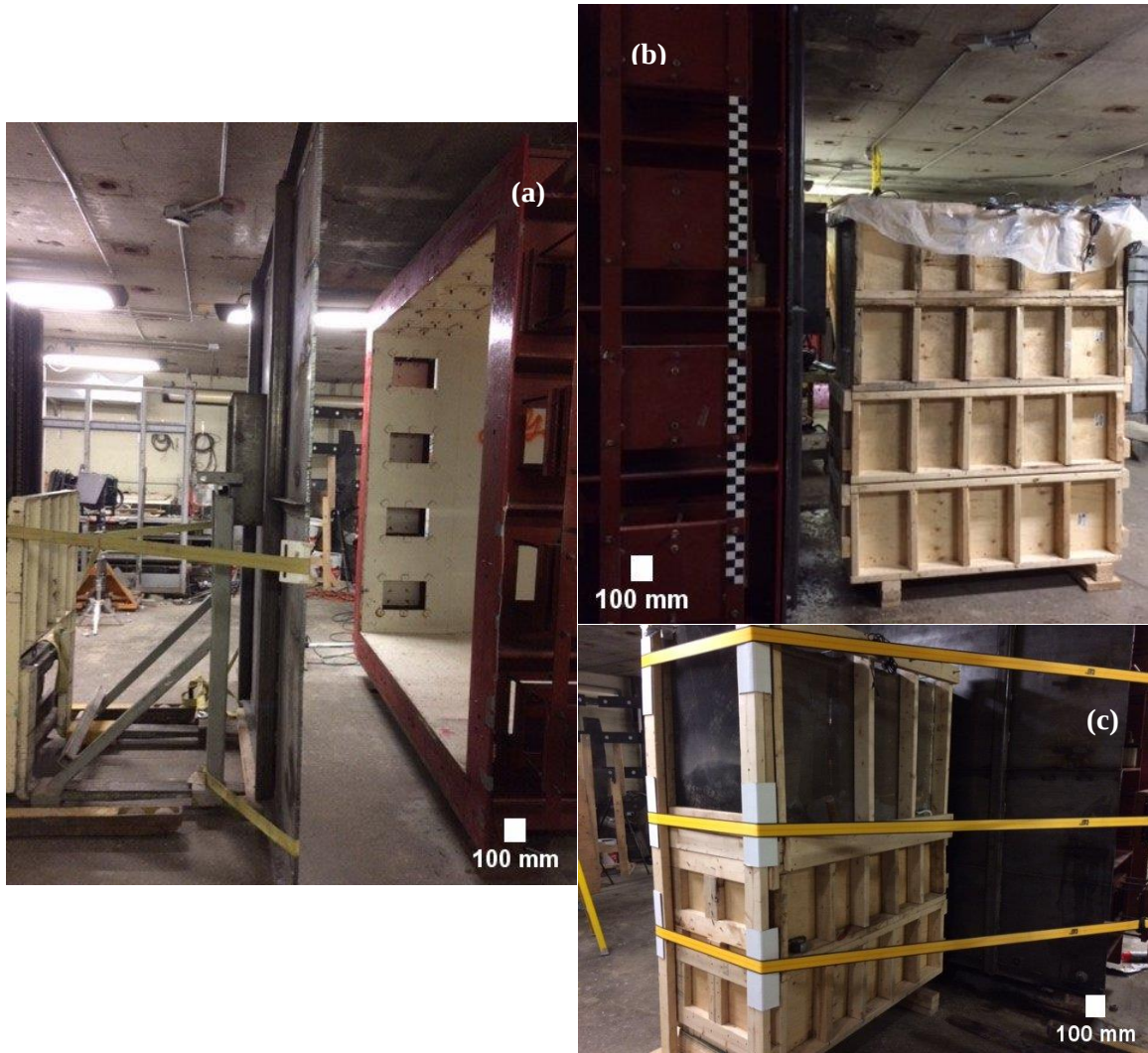
Figure 3.7-1: Test setup (a) covering the shock tube's mouth with a stiff plate; (b) placing the test specimen at the centre of the shock tube; (c) fastening the test specimen to the shock tube using straps
