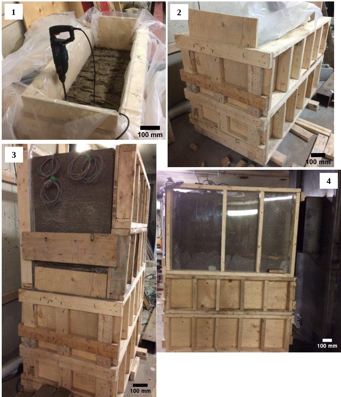
Figure 3.6: Steps of box preparation and soil compaction
