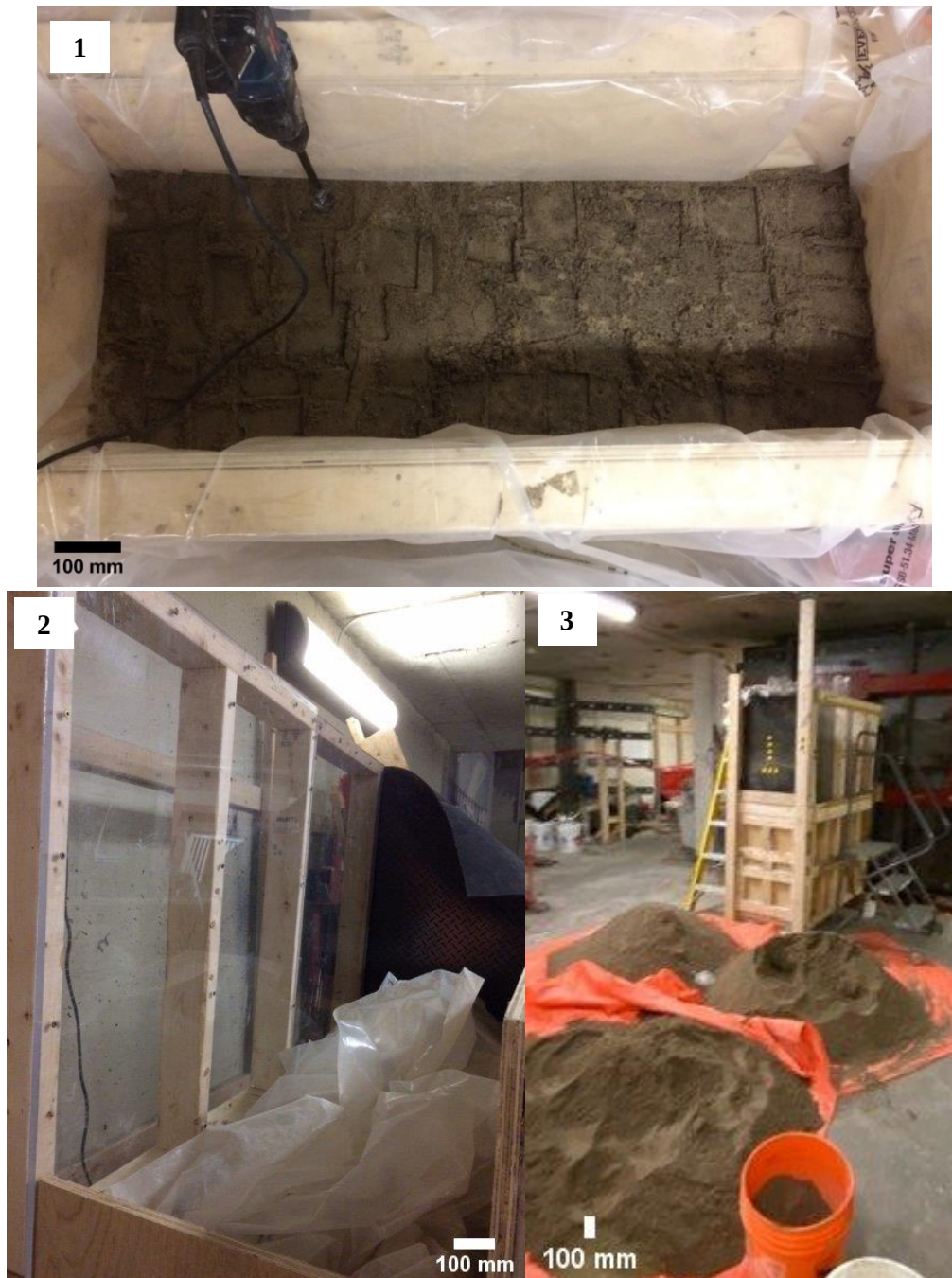
Figure 4.5: Steps of box preparation and soil compaction
