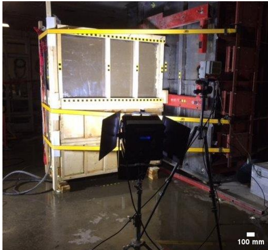
Figure 3.9: Test preparation at the Blast Research Laboratory of the University of Ottawa The test specimen was placed in front of the shock tube mouth, fastened with straps to prevent any movement during the blast test. The camera was facing the side view of the box, where the plexiglass was located, to capture sand particles movement.
