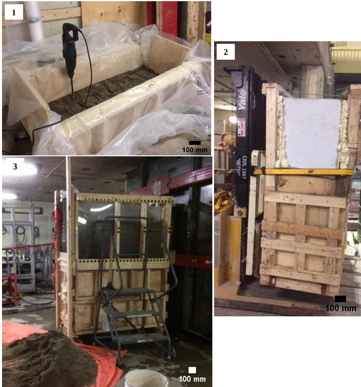
Figure 5.5: Steps of box preparation and soil compaction
