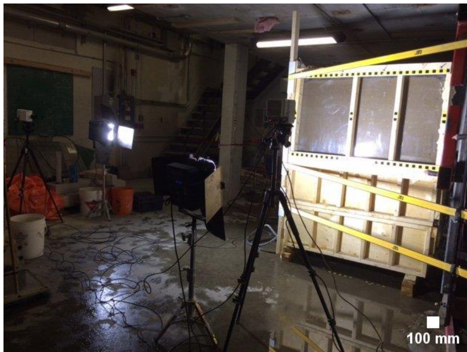
Figure 4.7: Test preparation at the Blast Research Laboratory of the University of Ottawa The test specimen was placed in front of the shock tube mouth, fastened with straps to prevent any movement during the blast test. The first camera was facing the side of the box, where the plexiglass was located, to capture sand particle movement. The second camera was facing the back of the specimen.
