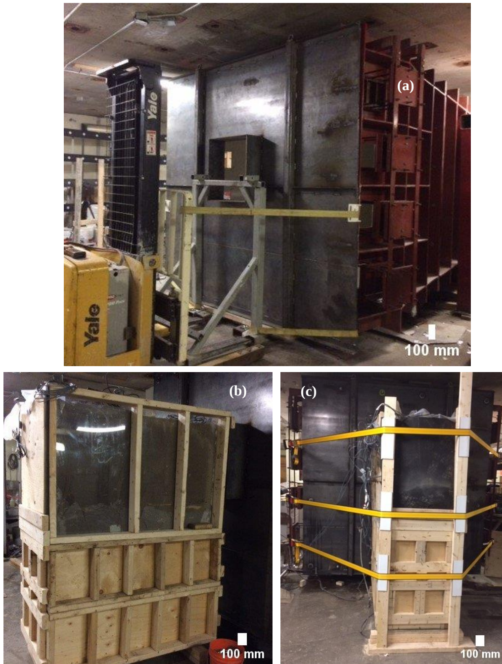
Figure 4.6-1: Test setup (a) covering the shock tube's mouth with a stiff plate; (b) placing the test specimen at the centre of the shock tube; (c) fastening the test specimen to the shock tube using straps
