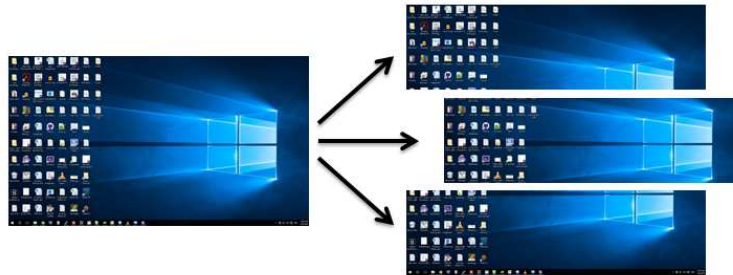
Figure 3.4: Revised OCR capture process, splitting fullscreen images into overlapping subtasks in parallel threads to reduce OCR execution time. There are always 2n - 1 slices produced, and in this case n = 2 .
