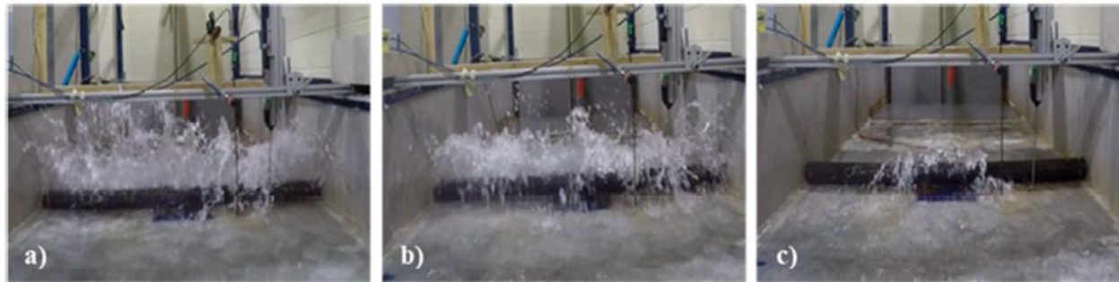
Figure 2.18. The impact of the bore for three upstream heights on the pipe: (a) 0.50 m, (b) 0.40 m, and (c) 0.30 m (Ghodoosipour et al., 2019b)
