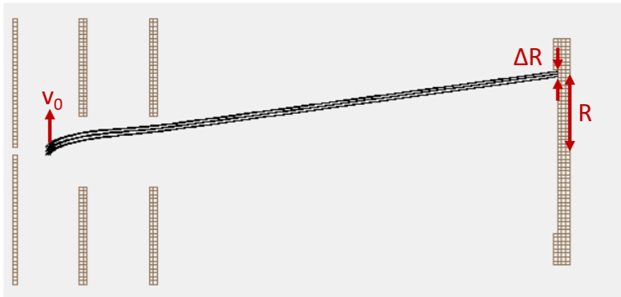
Figure 2.5: Schematic of how VMI energy resolution is calculated in simulation. Electrons with initial velocity v_0 follow trajectories (black lines) towards the detector with a spread \Delta R at a radius R from the center.
