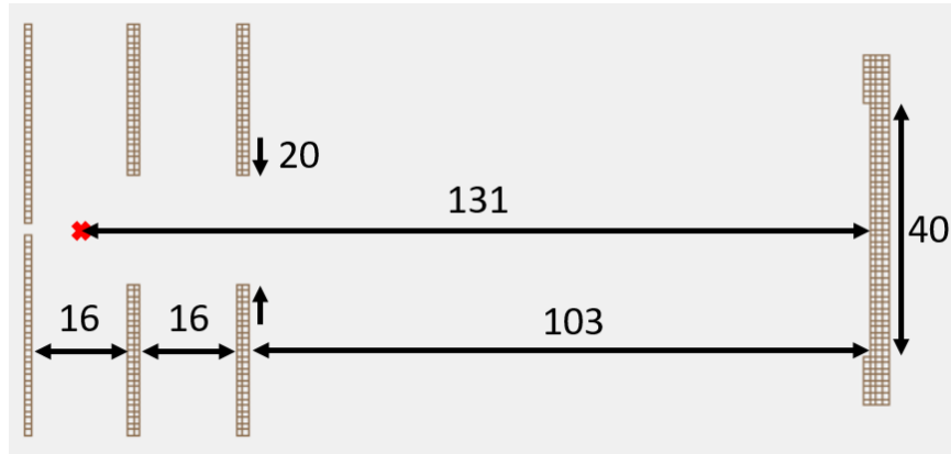
Figure 2.10: Dimensions of the 3 plate spectrometer used in SIMION simulations. The red cross indicates the interaction region. All units are in mm.
