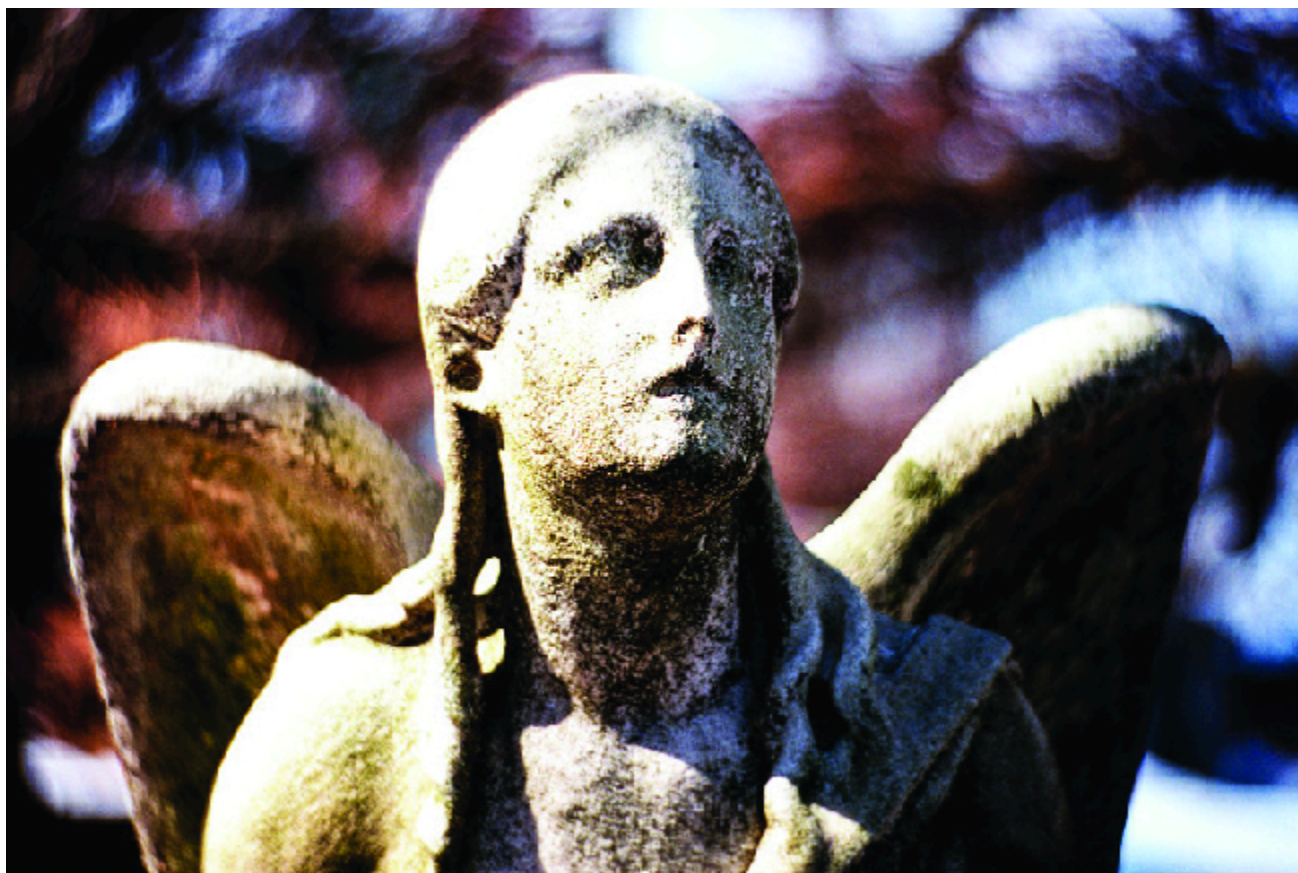
Figure 7.1.3. Statues made from carbonate compounds such as limestone and marble typically weather slowly over time due to the actions of water, and thermal expansion and contraction. However, pollutants like sulfur dioxide can accelerate weathering. As the concentration of air pollutants increases, the deterioration of limestone occurs more rapidly. (credit: James P Fisher III)
