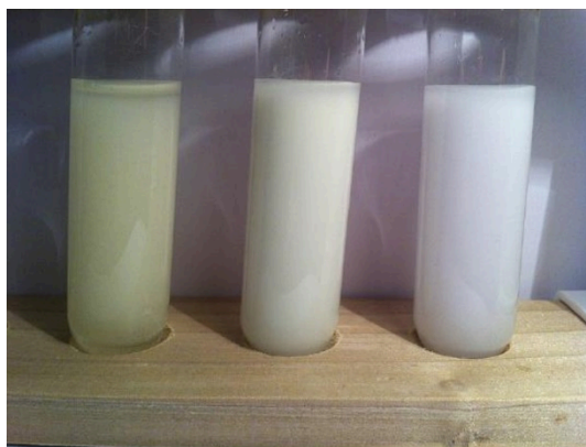
Figure 1.4.8. The three common silver halide precipitates: \text{AgI} , \text{AgBr} and \text{AgCl} (left to right). The silver halides precipitate out of solution, but often form suspensions before settling. Image used with permission (CC BY-SA 3.0; Cychr).
