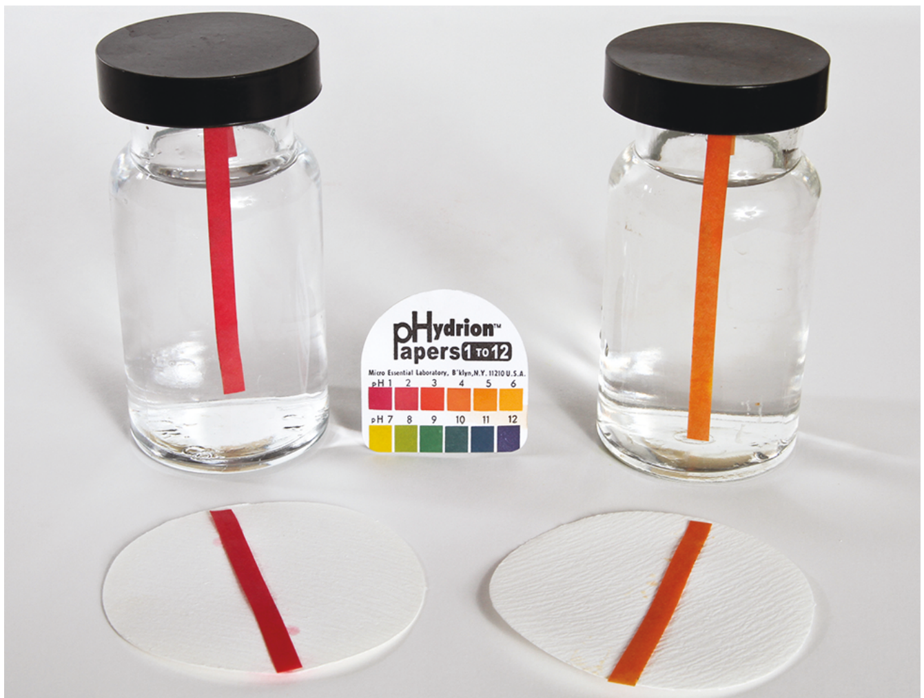
Figure 5.3.4. pH paper indicates that a 0.1 M solution of HCl (beaker on left) has a pH of 1. The acid is fully ionized and [\text{H}_3\text{O}^+] = 0.1 \text{ M} . A 0.1 M solution of \text{CH}_3\text{CO}_2\text{H} (beaker on right) is a pH of 3 ( [\text{H}_3\text{O}^+] =
