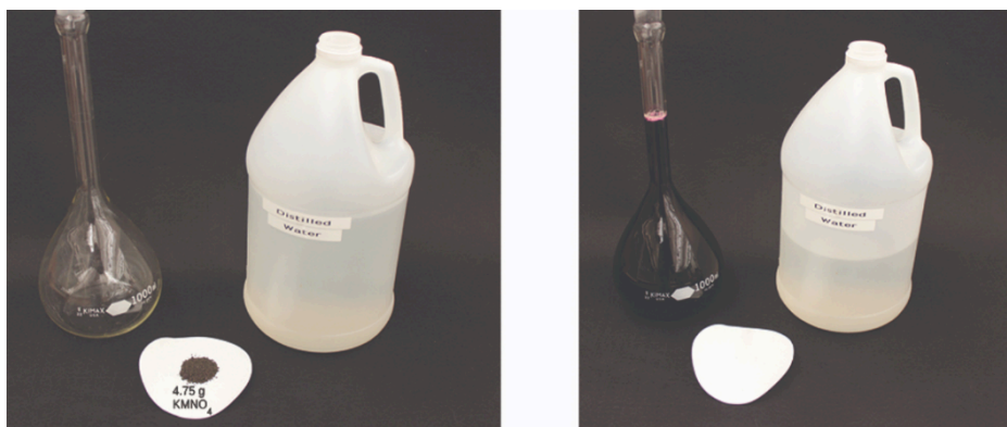
Figure 1.4.7. A solution of \text{KMnO}_4 is prepared by mixing water with 4.74 g of \text{KMnO}_4 in a flask. (credit: modification of work by Mark Ott)
