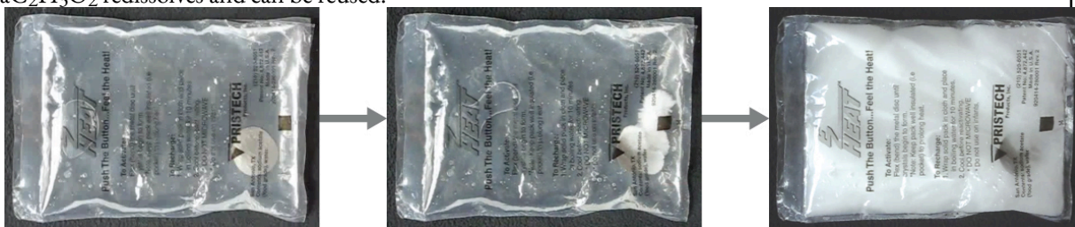
Figure 3.5.7. Chemical hand warmers produce heat that warms your hand on a cold day. In this one, you can see the metal disc that initiates the exothermic precipitation reaction. (credit: modification of work by Science Buddies TV/YouTube)
