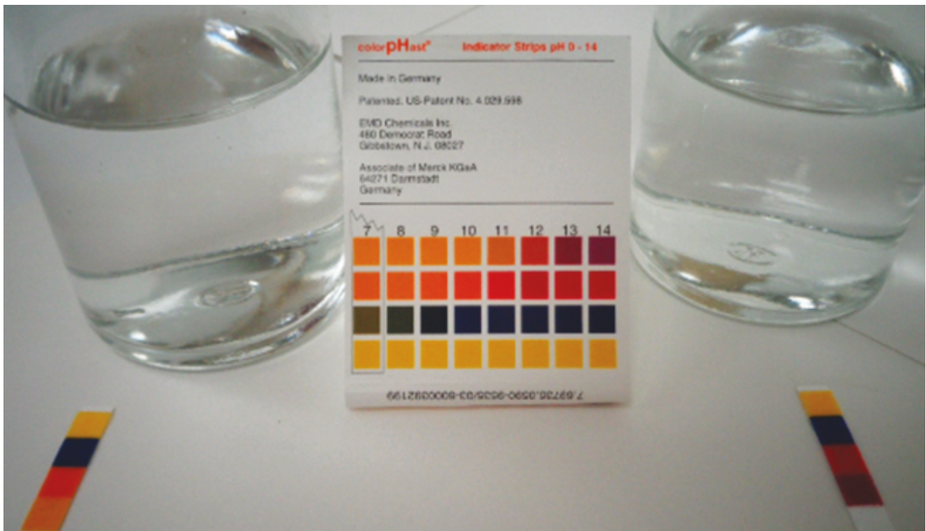
Figure 5.3.5. pH paper indicates that a 0.1 M solution of \text{NH}_3 (left) is weakly basic. The solution has a
