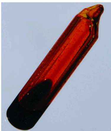
Figure 4.1.4. An equilibrium is pictured between liquid bromine, \text{Br}_2(l) , the dark liquid, and bromine vapour, \text{Br}_2(g) , the reddish-brown gas. Because the container is sealed, bromine vapour cannot escape and equilibrium is maintained. (credit: http://images-of-elements.com/bromine.php )
