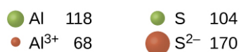
Figure 8.7.3. The radius for a cation is smaller than the parent atom (Al), due to the lost electrons; the radius for an anion is larger than the parent (S), due to the gained electrons.
