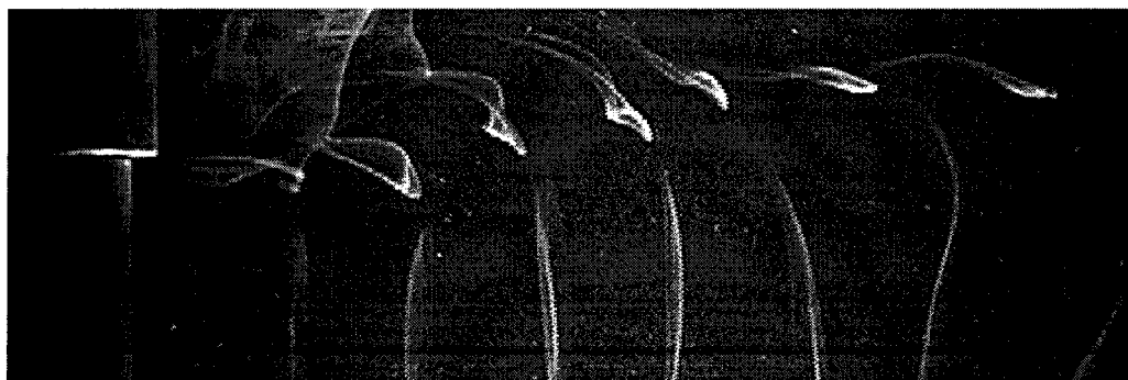
Figure 69: Shed vortices were bent in the streamwise direction until they formed half-loops. Double-step cylinder in uniform flow at Re = 118 .
