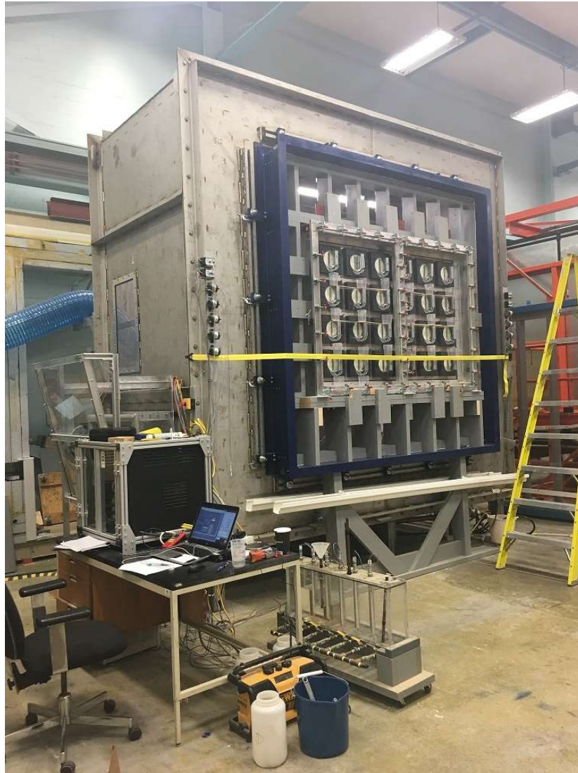
Figure 4.8 Dynamic wind and wall testing facility
