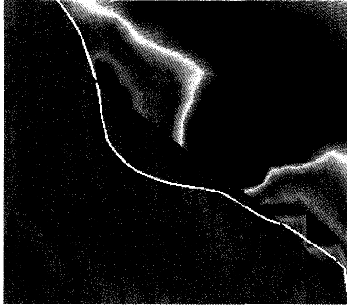
Figure 9.8: An example of a region belonging to \Omega_{\text{missing}} (in grey). Dirichlet boundary conditions are used on the black line and homogeneous Neumann boundary conditions are used on the white line.
