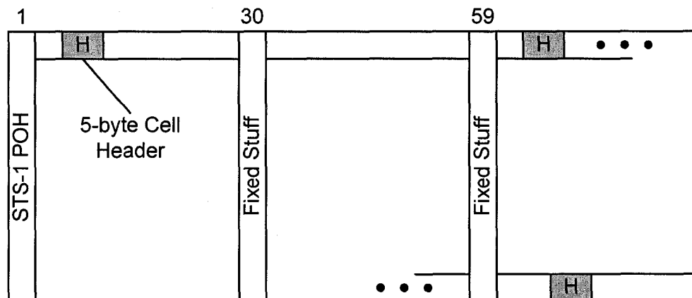
Fig. C.4: ATM Cell Mapping into a STS-1
