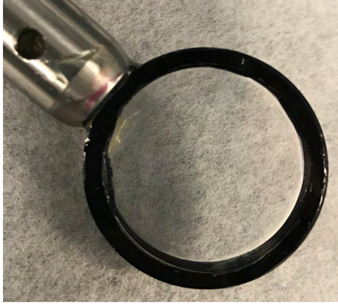
Figure 4.1: Photo of the airplate, our low-index spaceplate used in experiments.
