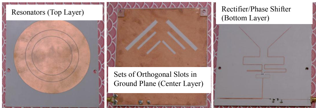
Figure 4 - Slot-Coupled Multi-resonator (Triband) [6]
