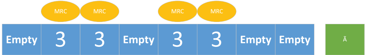
Figure 5.24: An example of the calculated \tilde{A} in the fourth scenario for N = 8 total subcarrier and M = 4 subcarrier per user.
