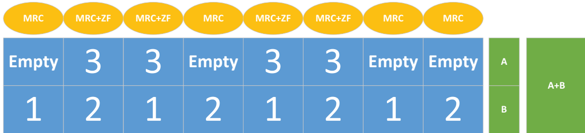
Figure 5.23: An example of the fourth scenario subcarrier mapping for N = 8 total subcarrier and M = 4 subcarrier per user.
