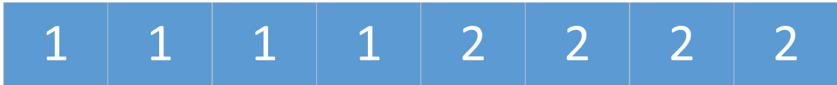
Figure 5.4: Localized subcarrier mapping for N = 8 total subcarrier and M = 4 subcarrier per user.
