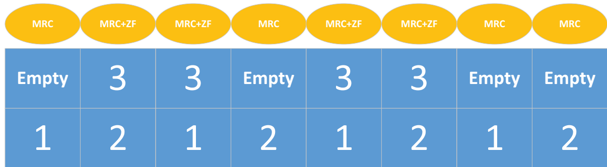
Figure 5.20: An example of the third scenario subcarrier mapping for N = 8 total subcarrier and M = 4 subcarrier per user.
