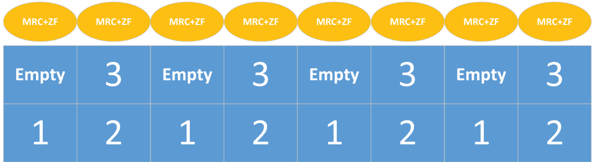
Figure 5.15: An example of the first scenario subcarrier mapping for N = 8 total subcarrier and M = 4 subcarrier per user.
