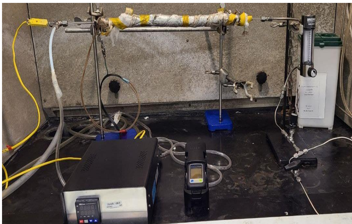
Figure 4.2 Schematic of SO 2 testing capture set-up
