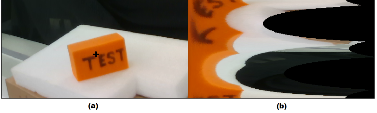
Figure 4.5: Example of polar image representation for fast level sets. (a) Image of object with estimated centre identified and (b) image warped to a polar representation.
