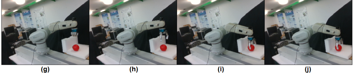
Figure 5.4: Images of the robot as it moves from the approach pose into the grasping pose and deforms the object. (g) Robot in approach pose with hand closed, (h) and open. (i) Robot in the grasping pose with fingers in contact with surface of the object, (j) and after deforming the object towards the desired shape.
