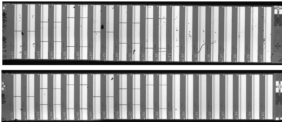
Figure 4-7 Microscope top view images of the fabricated laser devices on 2 bars, from the top L21-L40 (1500 \mu\text{m} ), L41-L60 (1250 \mu\text{m} )
