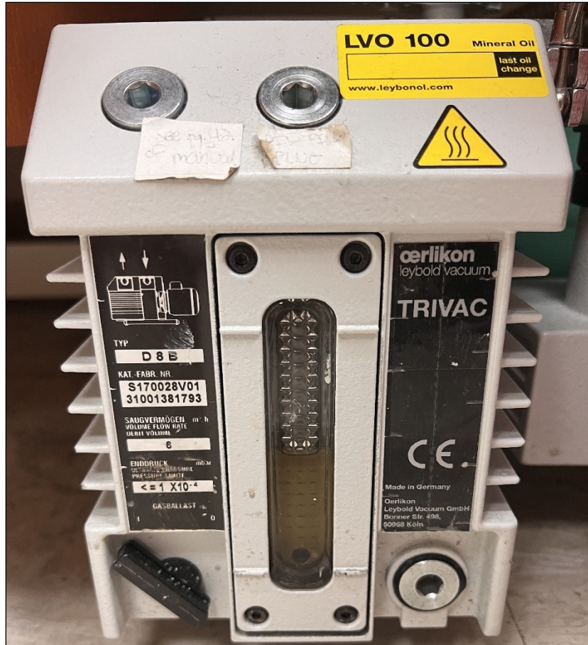
Figure A3. Flexcell vacuum pump. The bottom right plug is used to drain the LVO 100 oil. The plug directly above the oil line is used to refill the oil. The oil should be between the lines on the plate surrounding the oil level visualizer and should resemble the level shown above.
