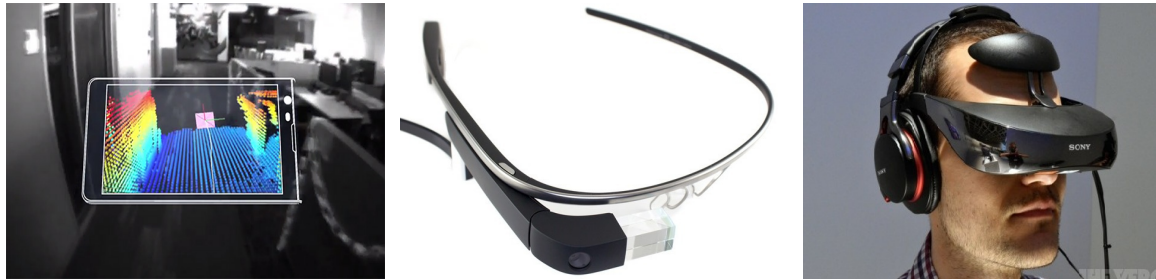
(a) Project Tango by Google (b) Google Glass project (c) Sony Head-mounted display
