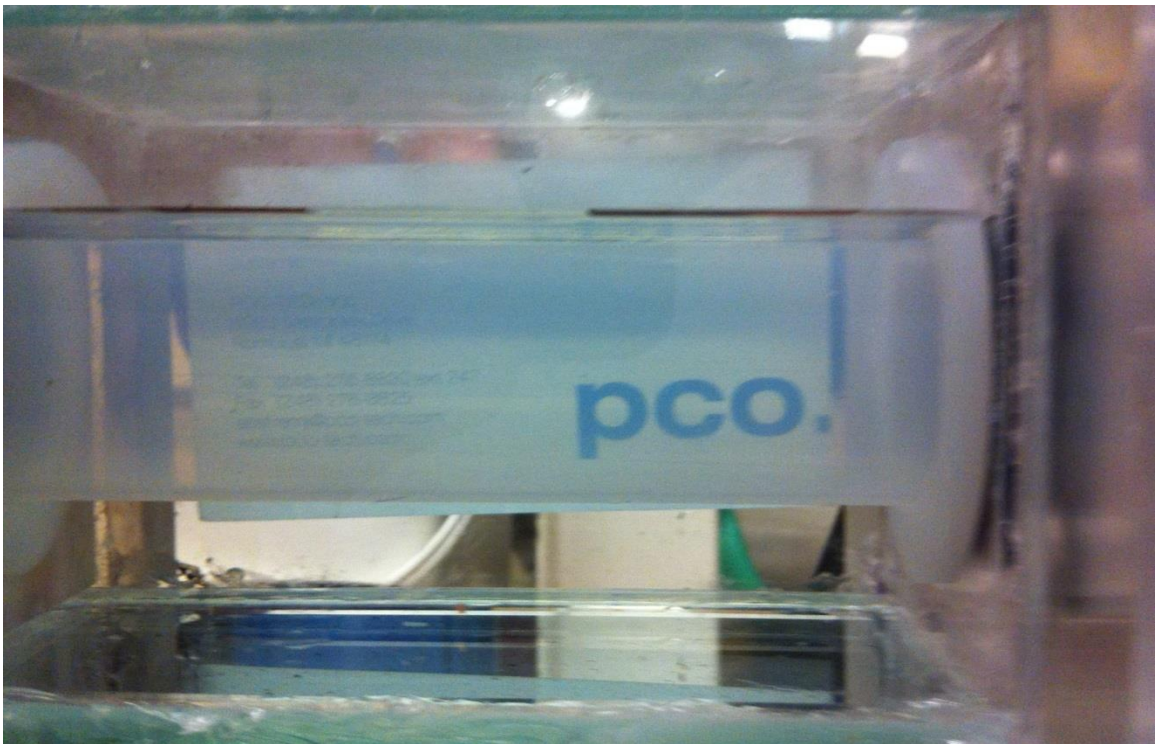
Figure 28: Undistorted view of a business card through the Teflon pipe section
