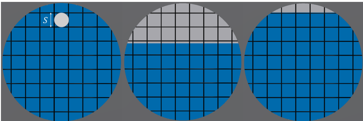
Figure 46: Examples of a sparse bubbly flow (left), and stratified flows (middle and right), which would be subject to large errors in void fraction measurement
