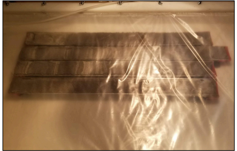
Photo 10: Core drying setup (cores)
