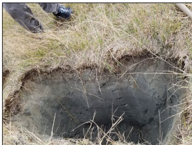
Photo 6: Test pit for horizontal cores
