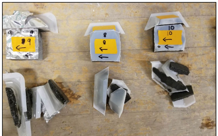
Photo 12: Thin sections prepared for cutting and polishing
