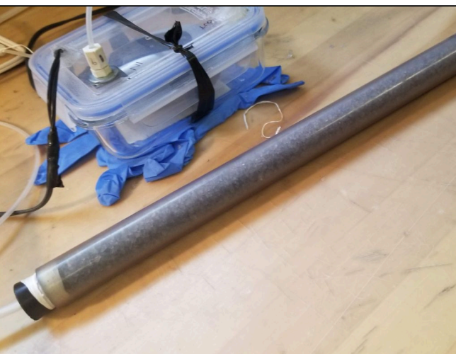
Photo 11: Core drying setup (dessicant)
