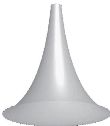
Figure 3.6: A pseudosphere is a surface of constant negative curvature.
