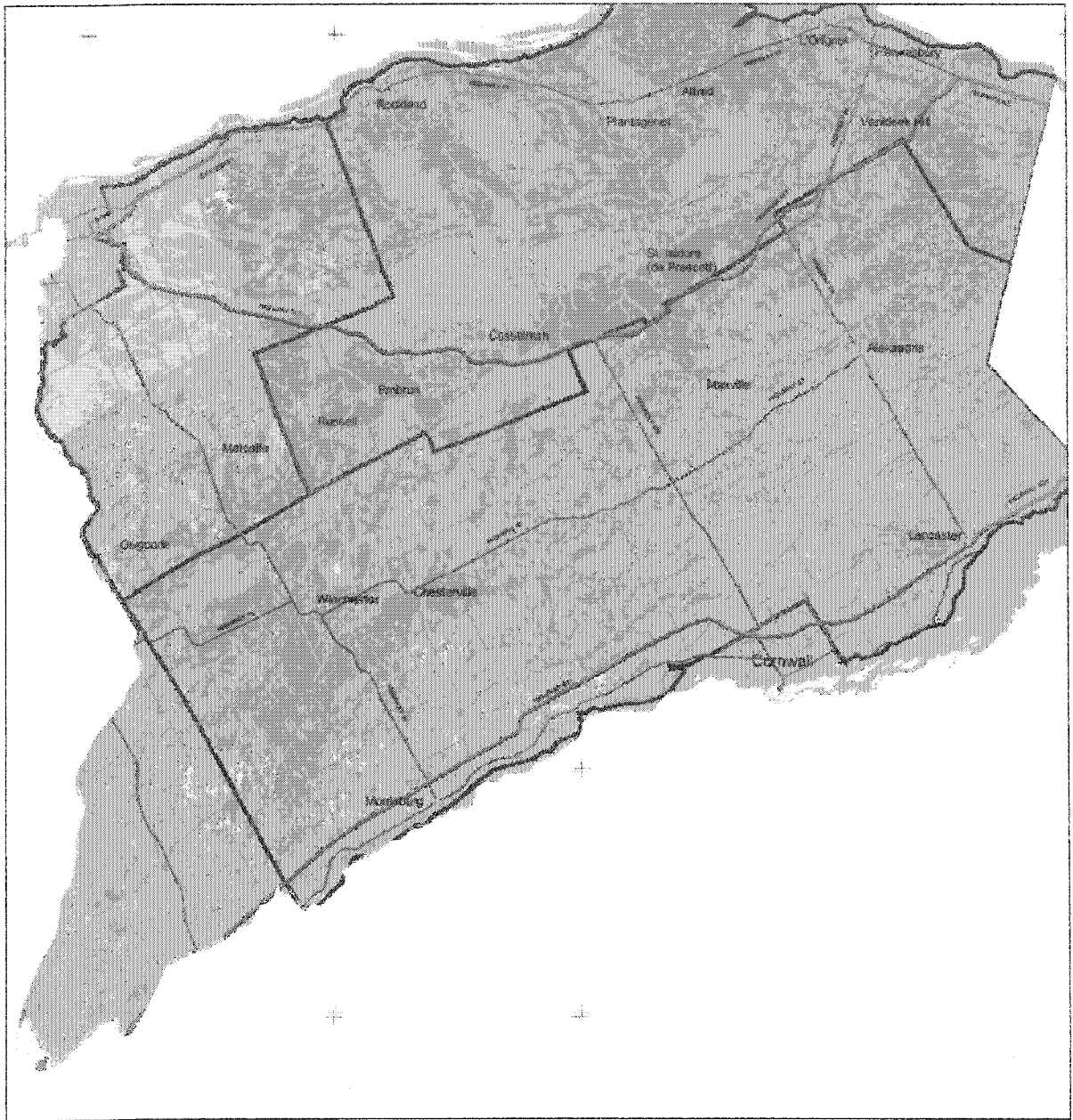
Figure 4: EOWRMS Soil type data used as spatial delineation of soil types for AnnAGNPS watershed model
