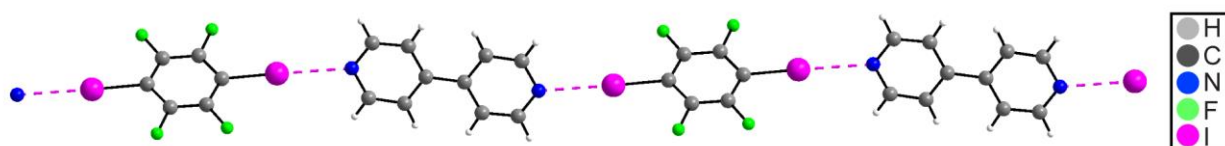
Figure 1.1.8. Depiction of the crystal structure of (1,4-diiodotetrafluorobenzene)(4,4'-bipyridyl) taken from Pennington and coworkers. 99 The dashed magenta line denotes the halogen bond. A legend of the atomic colors is shown on the right.
