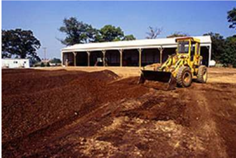
Figure 2.6 Composting by windrows (Elcock and Veil, 2005)
