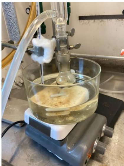
Figure 15. Vacuum sublimation apparatus used.
