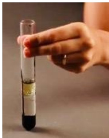
Liquids settle according to their weight
