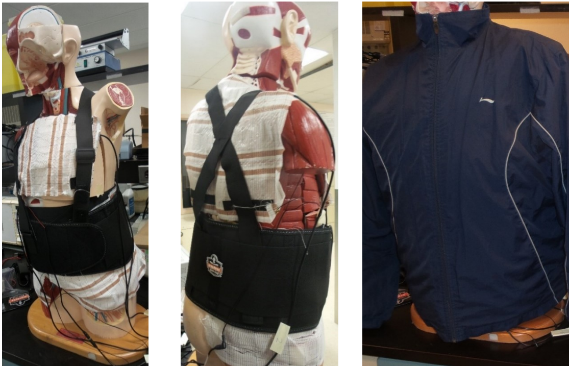
Figure 5-2 The manikin with the prototype of the electrical heating vest covered by a layer of outerwear
