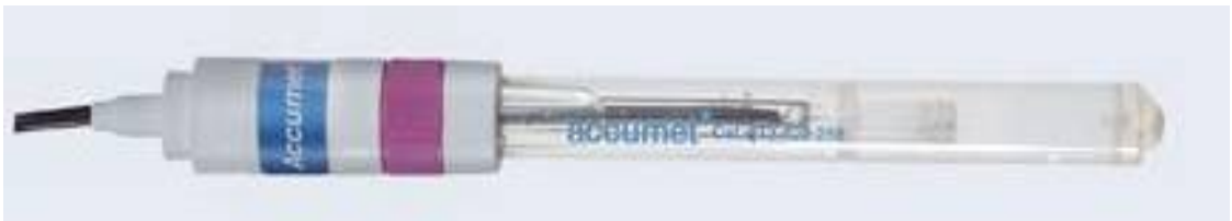
Figure 3-11: Saturated calomel electrode used as a reference electrode to measure corrosion potential (Fisher Scientific, 2012).
