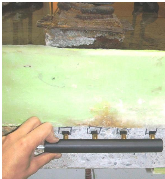
Figure 3-9: Daily monitoring of concrete electrical resistivity at specific locations.
