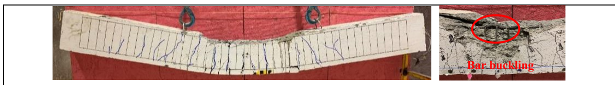
Figure A.63 Beam C100-No.5HS-DR-d/4 after the post-blast residual static test
