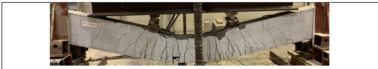
Figure A.87 Beam C100-No.5S1-DR-d/4 after the post-blast residual static test
