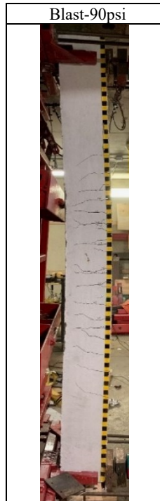
Figure A.89 Blast damage for beam C100-No.5S1-DR-d/4 (x1)
