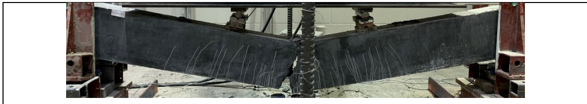
Figure A.133 Failure mode after the post-blast residual static test
