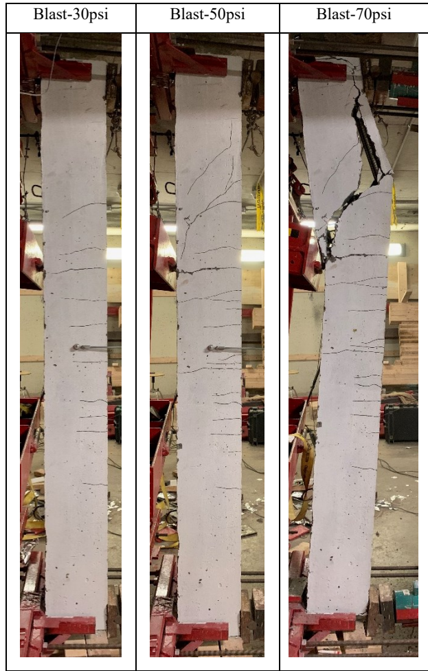
Figure A.79 Blast damage for beam CF100-No.5S1
