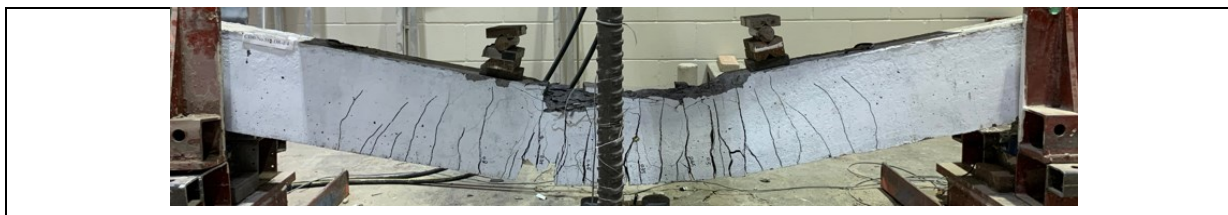
Figure A.99 Beam C100-No.5S2-DR-d/4 after the post-blast residual static test
