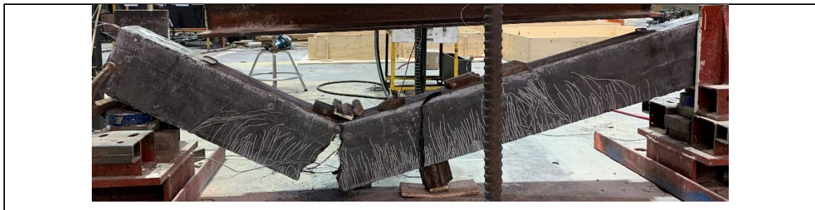
Figure A.127 Failure modes after the post-blast residual static tests
