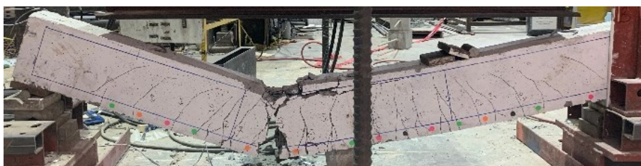
Figure A.59 Beam C100-No.4HS-DR-d/4 (x1) after post-blast residual static test
