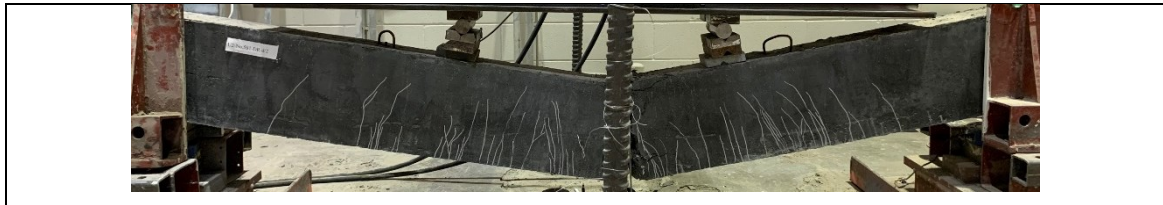
Figure A.137 Failure mode after the post-blast residual static test
