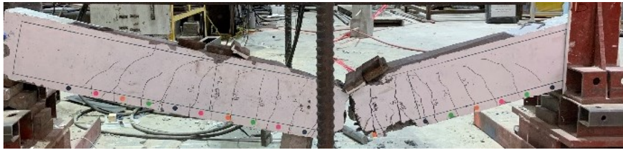
Figure A.55 Beam C100-No.4HS-DR-d/4 after the post-blast residual static test
