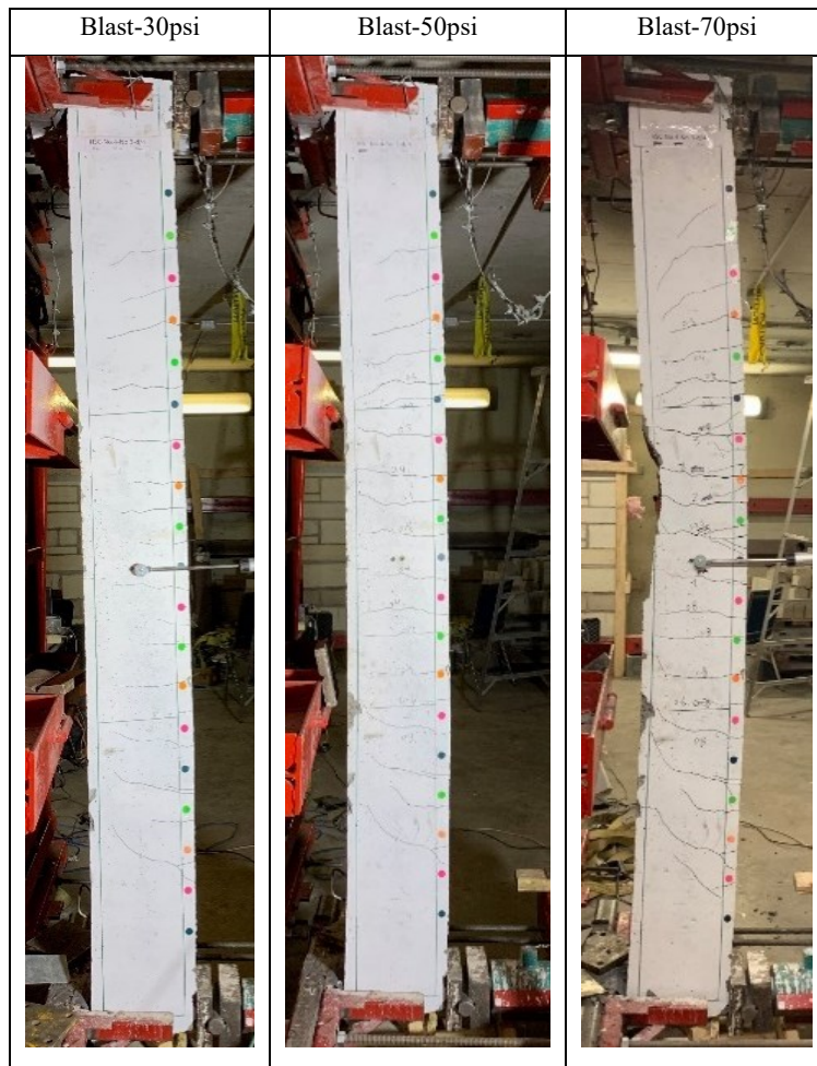
Figure A.52 Blast damage for beam C100-No.4HS-DR-d/4
