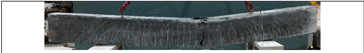
Figure A.117 Failure mode after the post-blast residual static test
