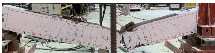
Figure A.71 Beam CF100-No.5HS-DR-d/2 after the post-blast residual static test
