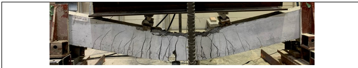
Figure A.83 Beam C100-No.4S1-DR-d/4 after the post-blast residual static test
