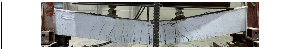
Figure A.95 Beam CF100-No.5S1-DR-d/2 after the post-blast residual static test
