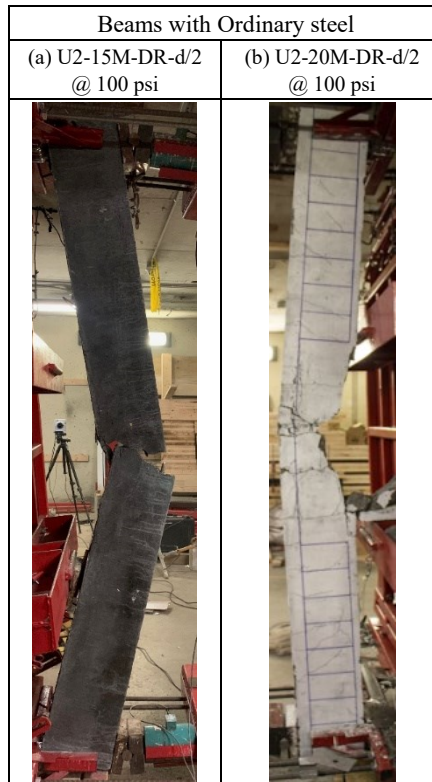
Figure 8.16 Effect of concrete type on failure mode in Group 2 (Ordinary steel)
