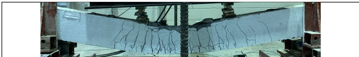
Figure A.91 Beam C100-No.5S1-DR-d/4 (x1) after the post-blast residual static test
