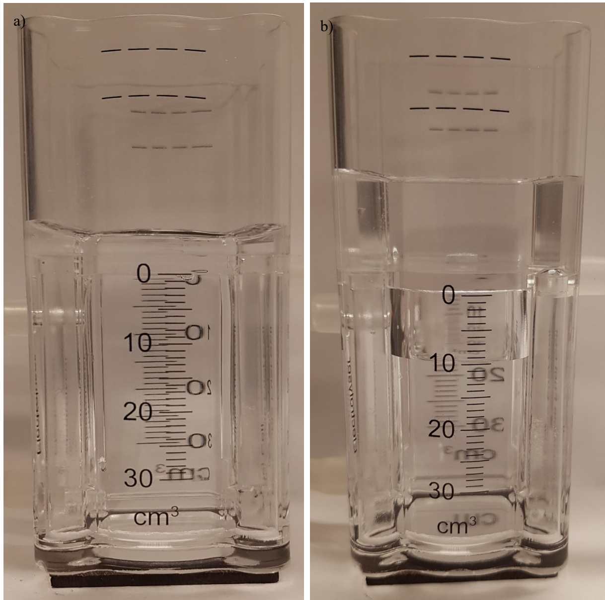
Figure 3.3.2: Water reservoir/gas storage tank for the PEM electrolyser, which was used to determine the volume of gas produced over a set period of time. The water reservoir/gas storage tank of the PEM electrolyser is presented a) with no hydrogen b) with 10 mL hydrogen.
